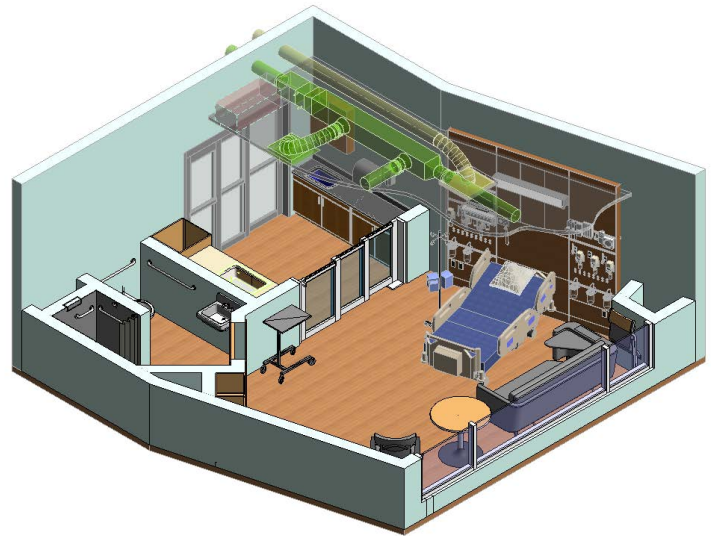
AHU zoning for emergency non-recirculation space
