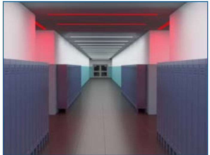
Luminaires adjacent to medical kits shall change to red or other specified color.
