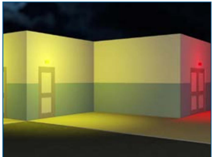
Figure 12 – Red lights flash at door nearest the danger; yellow lights flash at doors not adjacent to danger.
