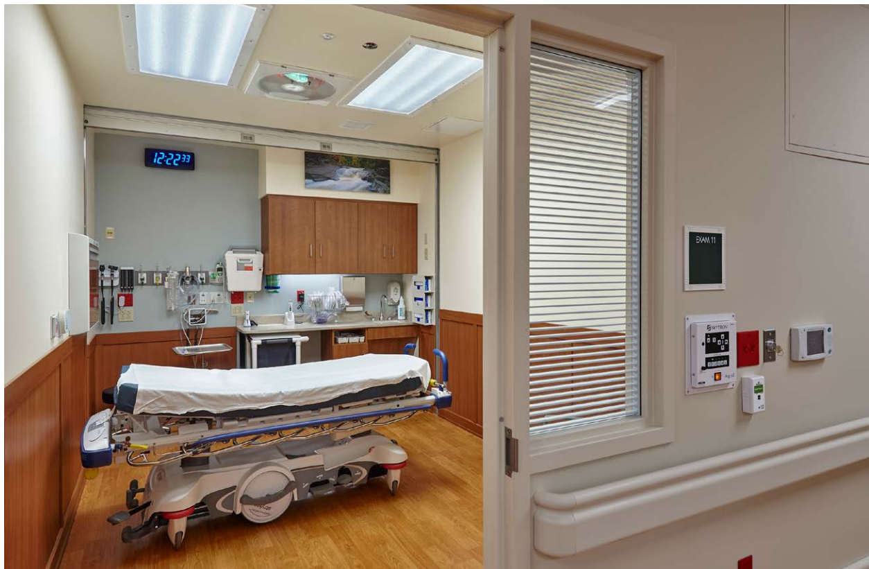
Emergency department exam rooms that can be converted to negative pressure can be used to separate patients with COVID-19 symptoms from those in need of critical emergency care.
