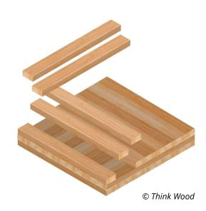
Cross-laminated timber (CLT) is the current industry buzz. It has been widely adopted throughout Europe and is making advancements in the U.S. To create, lumber board layers are stacked and glued at 90-degree angles and laid in odd lamination counts (three, five, seven, etc.). Alternating grains provide some two-way slab properties, though the odd lamination count does define a strong direction, or span direction.
