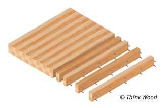
Nail-laminated timber (NLT) is one of the oldest types of mass timber and can be found in century-old buildings or bridge deck construction. NLT is created with pieces of 2x to 4x dimensional lumber ranging in thickness from 4" to 12" that are sandwiched together and then fastened with nails or screws. The commonly obtained materials and approach to construction means no manufacturing facility is required. Though you don't hear its name often, NLT is still in use today.
